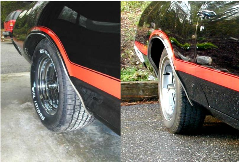
On the left is the new rubber, P295-50R15’s on 15 x 8” wide rims, on the right are the old P245-50R14’s on the original Olds 14 x 7” Super Stock I wheels. The new tires really fill the wheel well nicely while still allowing clearance to avoid rubbing.
