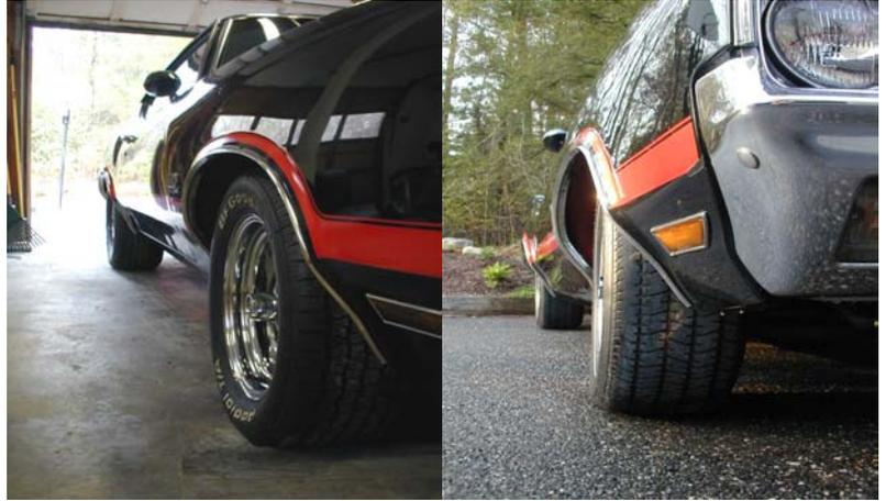
On the left is the new rubber, P265-50R15’s on 15 x 8” wide rims, on the right are the old P245-50R14’s . When going this wide in the front, extra care is required to make sure the tires do not rub the suspension or frame when turning at both full compression and full extension. These fit well and I have not see any rubbing at all.
